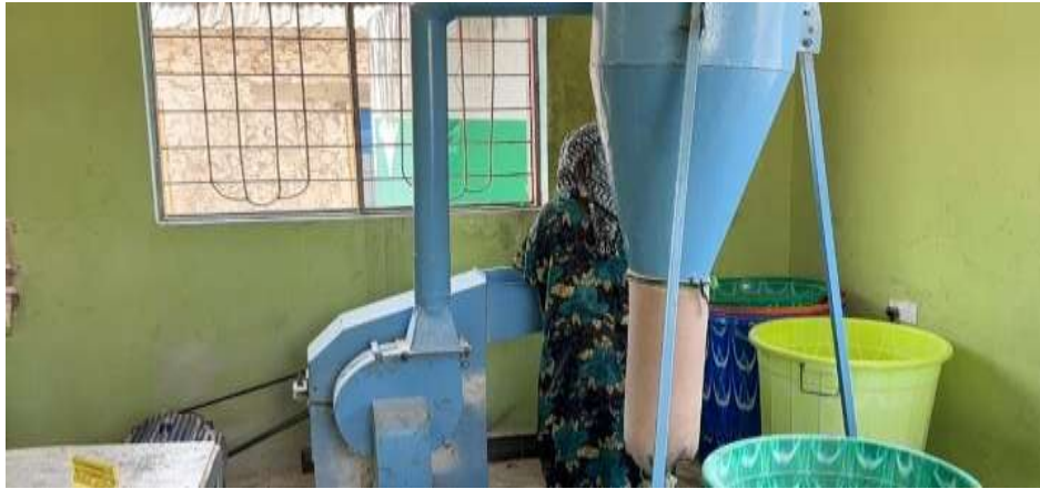
in the picture, machine used for making seaweed into seaweed flour
